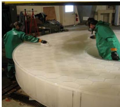
Figure 1: Final acid wash of primary mirror.
